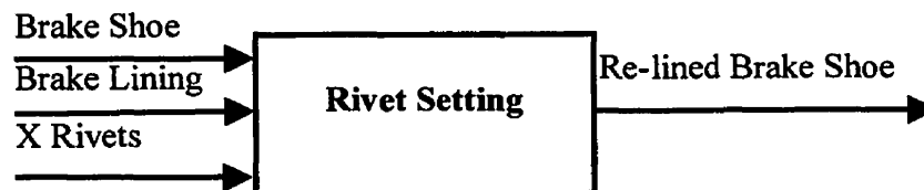
Figure 5-14 Overall functionality of rivet setting tool (adapted from Hubka et al ,1988)
