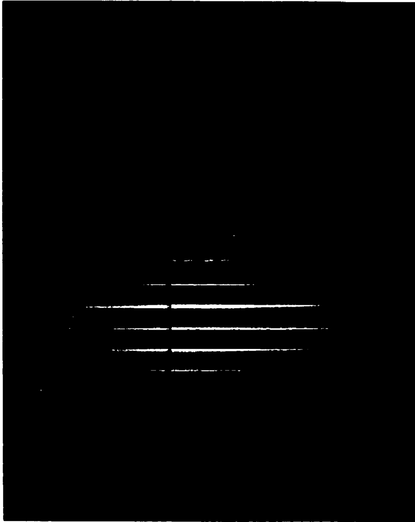
Figure 5.6: A sample preprocessed frame of M31 globular cluster B124 obtained with the MOS/ARGUS setup at CFHT. The dispersion axis is horizontal. Refer to Figure 5.5 for a frame layout schematic. Cosmic ray events are evident as small bright specks in the image.
