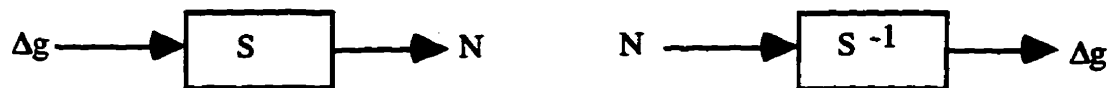
Fig. 3-2: Two examples of single-input single-output systems: Stokes' and inverse-Stokes' integrals, N is the geoid height, \Delta g is the gravity anomaly, S and S^{-1} are Stokes' and inverse-Stokes' kernels, respectively.
